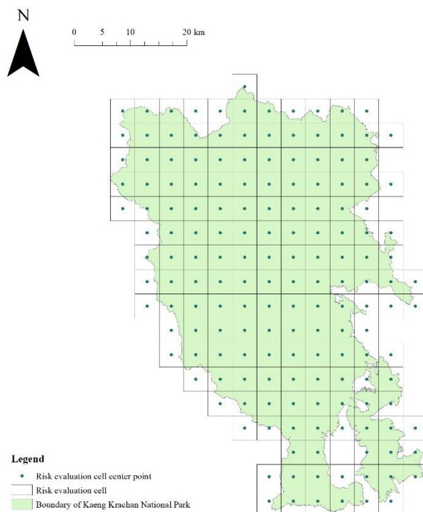
Figure 2. The spatial representation of the grid cell matrix with 5\text{km} \times 5\text{km} size cells, bordering the Kaeng Krachan National Park
